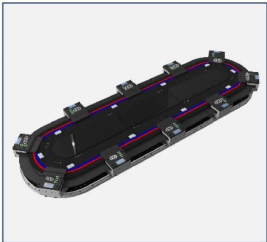
Wireless power supply magnetic drive line
